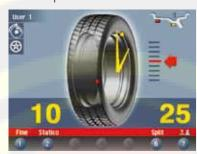
ALU-S balancing mode (adhesive weights on the internal rim planes) with specific counterweight position indicator (position repeater)
