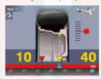
Eccentricity measurement with sonar (1st Harmonic and Peak to Peak) Automatic and quick eccentricity measurement during the normal balancing cycle
