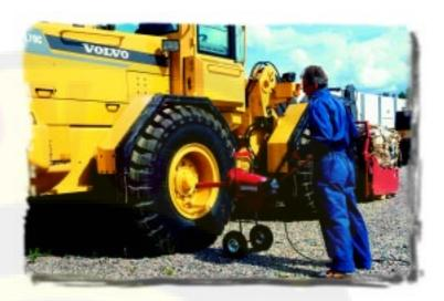
The *COLUMBUS* electric wheel nut runner operates at extremely high force. The machine is equipped with a rotary flywheel which delivers all of its energy to the nut in the form of an impact. The machine socket tube is provided with one inch square socket drive for power sockets. An ingeniously designed spring system makes the machine body almost weightless, minimising the effort required to adjust the height.
