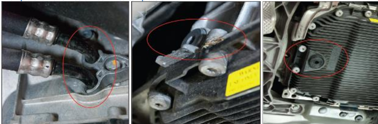
Delivery and return pipes, level indicator, drain plug
