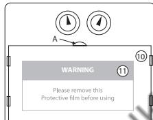
The internal protection screen (10) is removable by sliding it down by placing a finger on (A).
