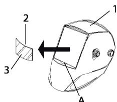
The outer protection screen (2) can be removed by placing a finger under the screen on (A) of the helmet (1).
