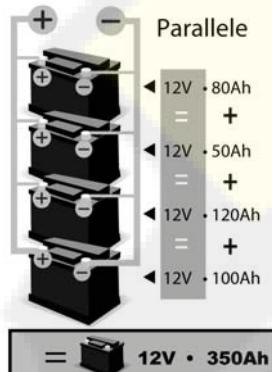
Several batteries can be charged simultaneously by connecting them in parallel (the + terminals connected to the red clamp and the - terminals connected to the black clamp). These batteries or grouped batteries must be at the same voltage 12V or 24V.
